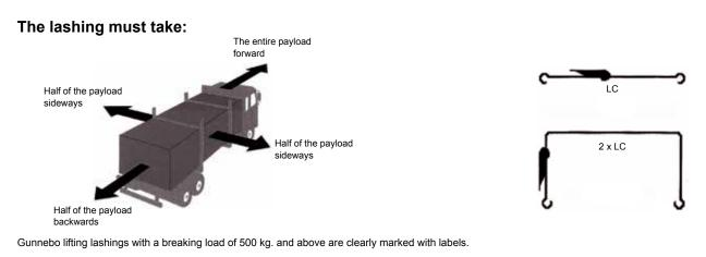
The dimensioning af a lashing arrangement must be based on local regulations.
